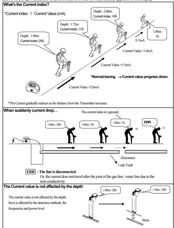
Each time a Depth calculation is taken, a Current Index simultaneously appears on the display.
