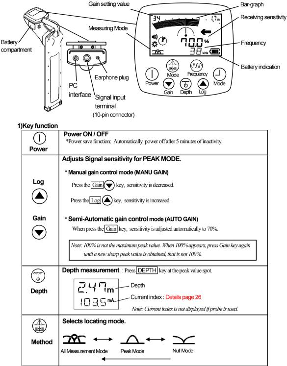
All Measurement Mode: Maximum sensitivity is the point directly above the object
